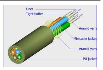
The tight-buffer in both cable options is made of a rugged material specifically designed for tactical cables. The minicable and outer jackets are extruded of polyurethane.
